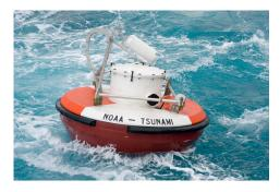
The International Tsunami Warning System monitors oceans through a network of buoys and scientific instruments. When the instruments detect a major earthquake and the potential for tsunami to occur, warnings are issued to local authorities who can order the evacuation of low-lying areas if necessary.
